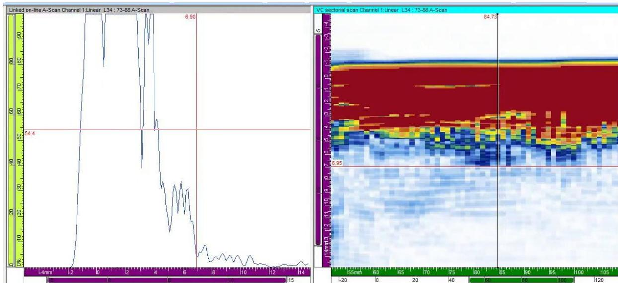
Next set of pictures shows the results of 1mm FBH at a depth of 5mm using DDF. The defect can be seen clearly and has good separation from the interface echo. There is marked improvement in the signal strength as can be seen in the A-Scan. Increasing both the amplitude and sizing resolution.
