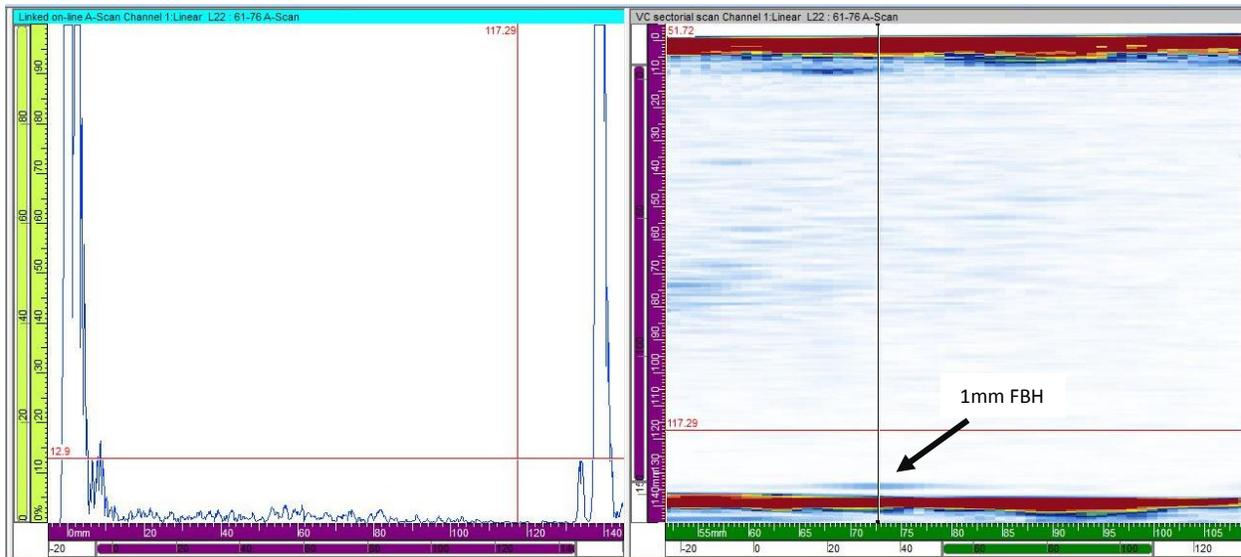
For every depth in the experimental setup the maximum amplitude of defect response in recorded with and without DDF. Two independent experimental runs are performed for measurement of amplitude to consider the effect of experimental fixture's variation.
