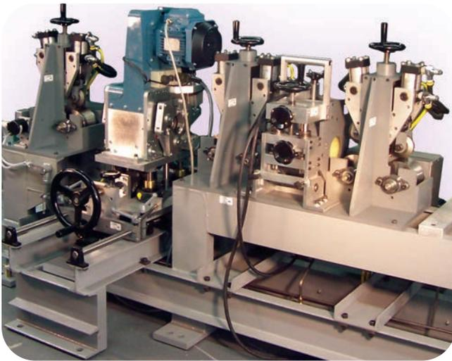
*Above is a picture of one of many test configurations provided by MAC. This system consists of an encircling eddy current rotary and an ultrasonic rotary mounted on a dual pinch "V" Roll bench. In this instance, long, continuous seam type surface defects as well as subsurface and internal defects are being detected.*
