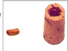
In order to calibrate the equipment, metal filings are placed inside of a cork to simulate an inclusion.
