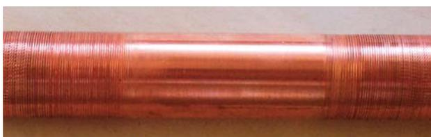
Tubes tested are for heat exchangers and mounted in shells in which you can find several support plates. Therefore tubes can have different lengths and different number of lands (lands are areas with no fins, fitting in the support plates).
